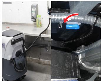
2. Fill the tank with a clean water. The clean water temperature must not exceed 40 °C.
