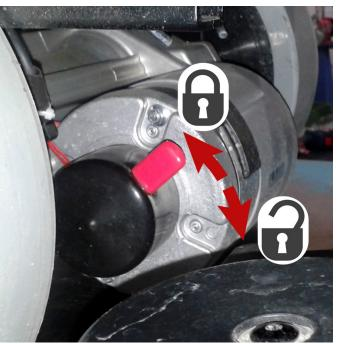
Check if the electromagnetic brake is locking.
