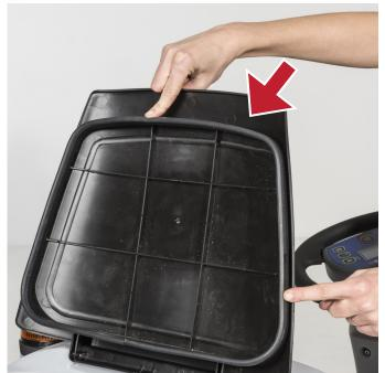
Check the lid gasket is in good and working condition and sealing when lid is closed.
