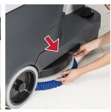
2 Check if the brush are correctly installed and not worn out or if there are external materials avoiding brush rotating.
