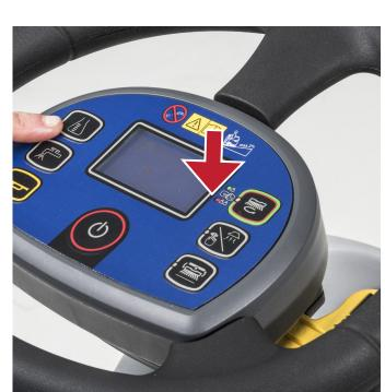
3 Check if the green switch Led of the One-Touch button is flashing. Wait until the light is steady.
