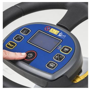
Restart the machine without pressing the drive pedal.
