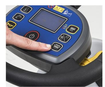
16. Press the click-off button and wait for the brush/pad holder to fall on the floor. Remove to clean or change brush.
