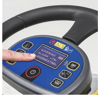
1 Check if there isn't any brush motor 2 overload "WARNING ALARM F2" on the display.
