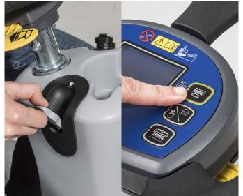
6. Insert the operator key, then start the machine by pressing the One-Touch button.
