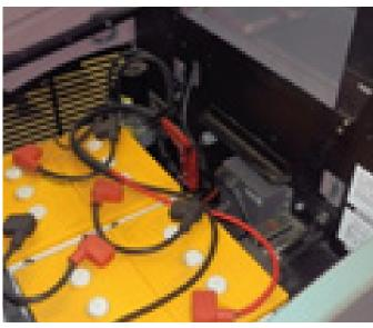
2. For the battery version check the battery voltage and charge if needed.
